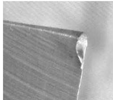
**Figure 5: Severe Flank Wear on Tool**
