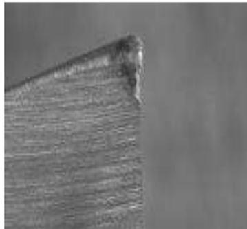
**Figure 4: Medium Flank Wear on Tool**
