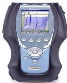
Figure 1: Field paq Vibration Analyzer
