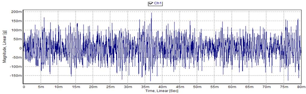
Figure 9: Amplitude-Time Spectrum of Medium Wear Condition (0.3 mm Flank Wear)
