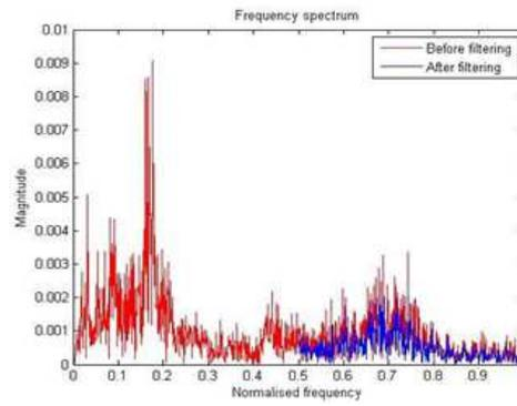
Figure 13: Filtering of Signals above 5 Khz Using Filter
