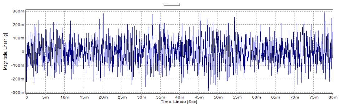
Figure 12: Amplitude-Time Spectrum of Severe Wear Condition (above 0.6 mm Flank Wear)
