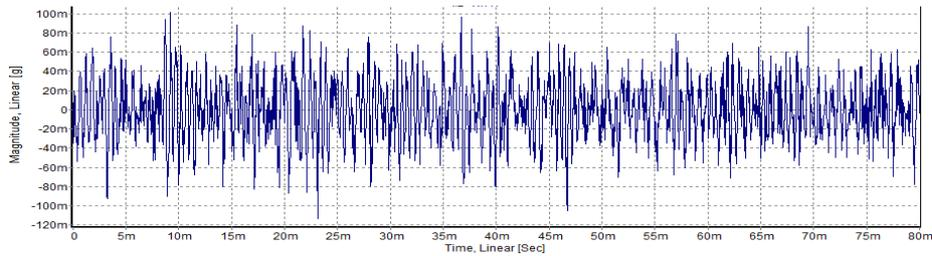
**Figure 6: Amplitude-Time Spectrum of Initial Wear Condition**
